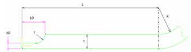
(a) Cross-section of the 'new-shape' for the slot wedge
