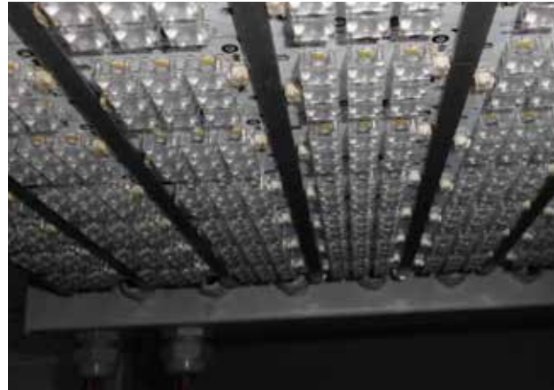
Figure 1 - Light engine seen under an angle from the measuring plane, where the module is placed
