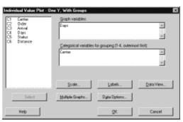
The list box on the left shows the variables from the worksheet that are available for the analysis. The boxes on the right display the variables that you select for the analysis.
