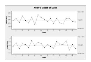
The  $\overline{\mathbf{X}}$  and  $\mathbf{S}$  chart now includes the new subgroup. The mean ( $\overline{\mathbf{X}} = 2.978$ ) and standard deviation ( $\overline{\mathbf{S}} = 0.6207$ ) have changed slightly, but the process still appears to be in control.
