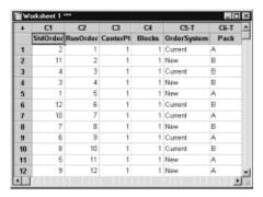
The RunOrder column (C2), which is randomly determined, indicates the order in which you should collect data. If you do not randomize a design, the StdOrder and RunOrder columns are the same.
