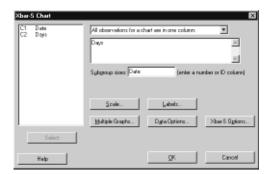
7 Click **Xbar-S Options**, then click the **Tests** tab. Notice this dialog box reflects the tests and test values you specified earlier. (See *Set options for control charts* on page 4-2.)
