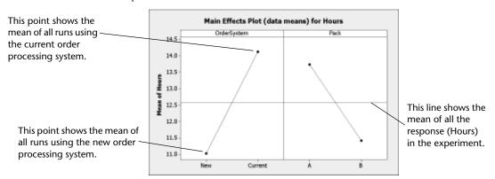
The order processing system and packing procedure have a similar effect on order preparation time. That is, the line connecting the mean responses for the new and current order processing system has a slope similar to slope of the line connecting the mean response for packing procedure A and packing procedure B. The plot also indicates that orders using:
