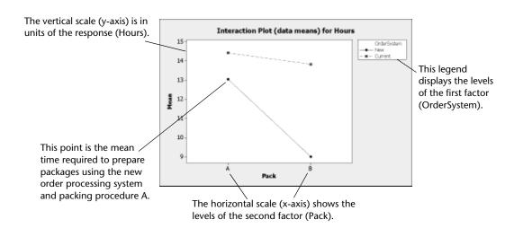
An interaction plot shows the impact that changing the settings of one factor has on another factor. Because an interaction can magnify or diminish main effects, evaluating interactions is extremely important.
