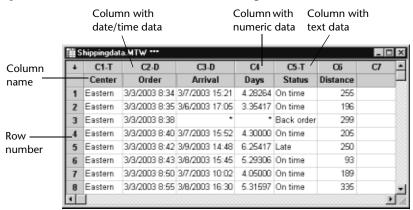
MINITAB accepts three types of data: numeric, text, and date/time. This worksheet contains each type.
