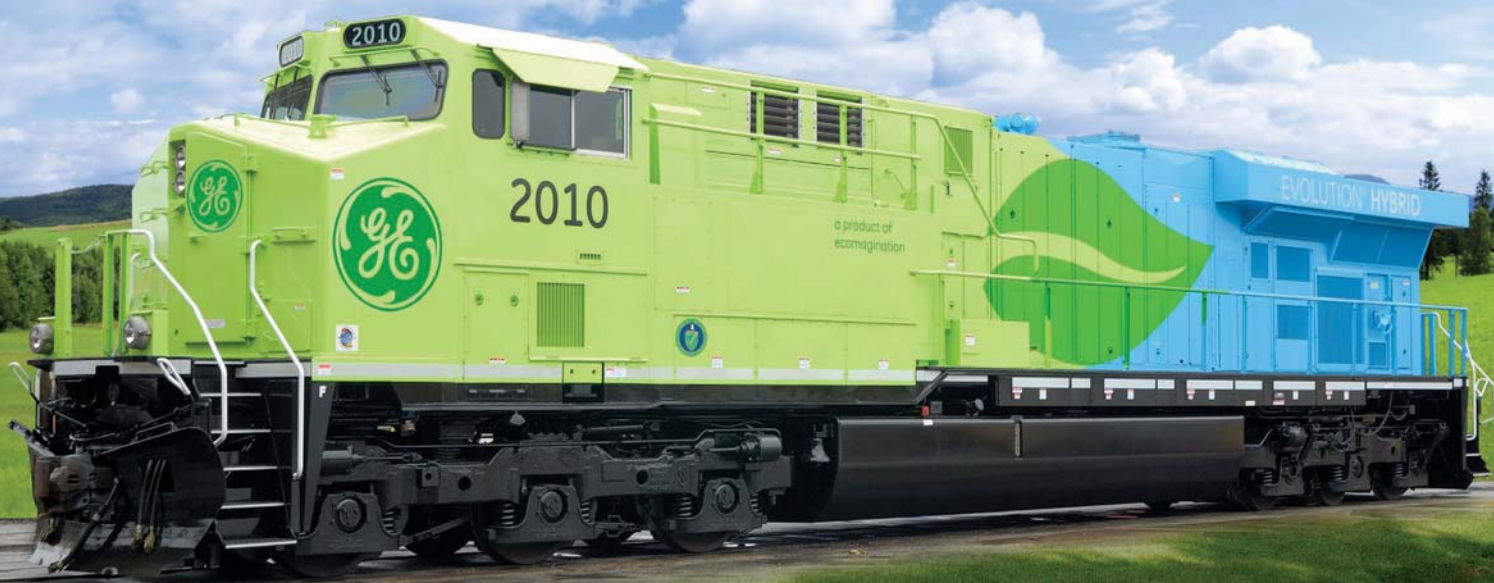
General Electric's Ecomagination SM technology is exemplified by the Evolution ® Hybrid Locomotive. GE will utilize batteries to help power these locomotives. Photo courtesy of GE Transportation.
