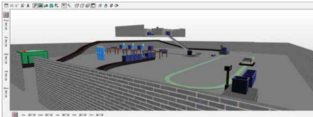
Figure 20: A Quick3D view of a manufacturing layout – multi floors, conveyor elevations, etc.
