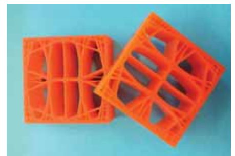
FIGURE 1. Top: Geometry of a unit cell. Middle: Simulation results showing mechanical stress for an optimized design with one planar direction having half the stiffness of the other. Bottom: 3D-printed samples.
