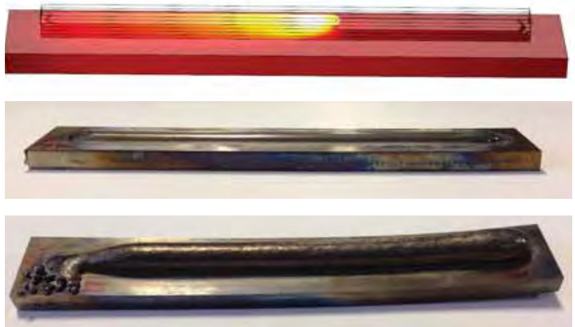
FIGURE 2. During the SMD process, thermal cycling induces residual stresses on the manufactured parts. Top: Simulation of the SMD part. Middle: The part after just one deposited layer, with no noticeable deformation. Bottom: After six deposited layers, deformation is visible to the naked eye.
