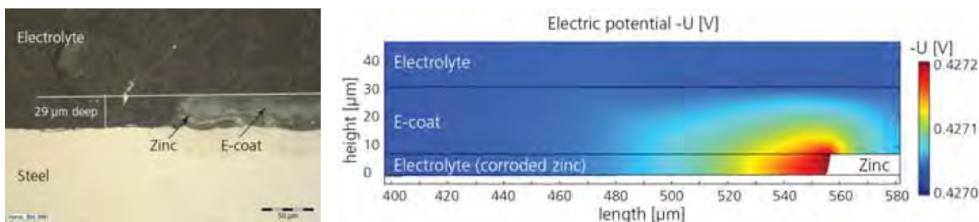
FIGURE 5. Left: Close-up of a cross-section of the test sheet where a scratch has destroyed part of the e-coat and zinc layers. Right: The COMSOL Multiphysics® software results showing the electric potential in the e-coat and electrolyte. The white region indicates the remaining zinc after much of it has already been consumed.
