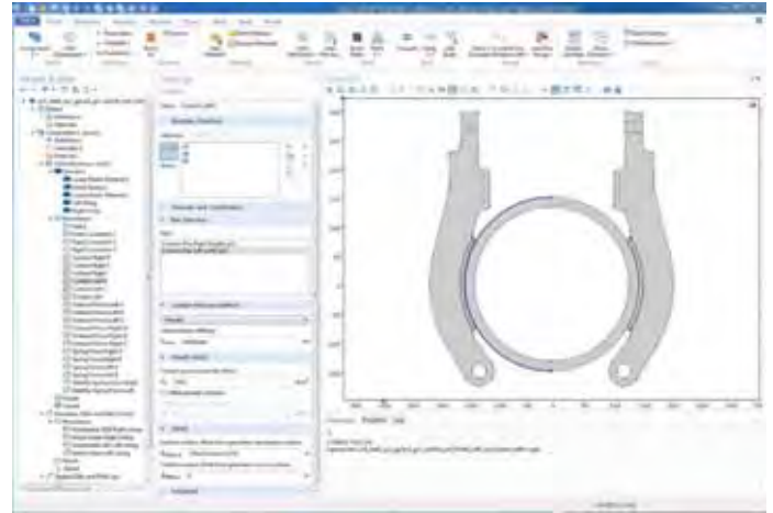
FIGURE 3. COMSOL Multiphysics® software model used to calculate brake lining wear.
