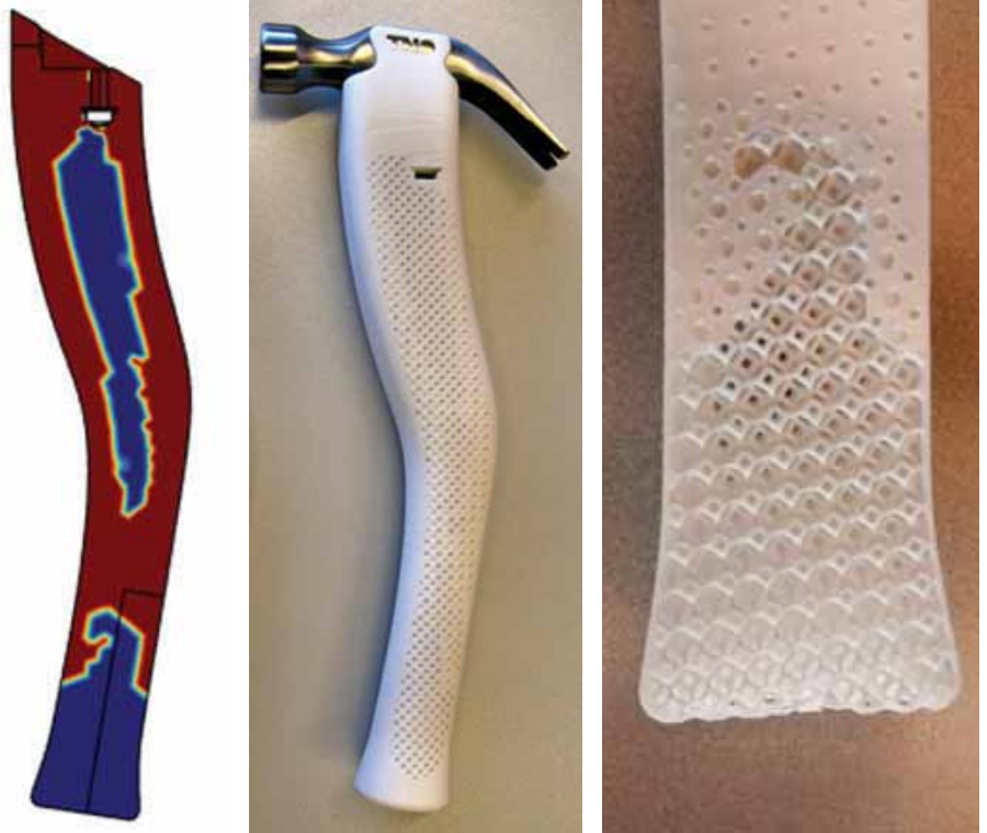
FIGURE 5. Left: Topology optimization result in the COMSOL® software. Center: The optimized hammer handle, printed in nylon. Right: Close-up of the pattern containing three different cell types: most dense cells with small holes near the top, least dense cells toward the bottom, and a few intermediate shapes in between.
