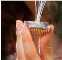
Fluid-Screen (formerly Alpha-Screen) brings the functionality of a lab to a small portable device that fits in the palm of your hand and detects bacteria from blood and water in less than 30 minutes. Fluid-Screen uses a patented electric field and biosensor technology to rapidly collect and detect bacteria.
