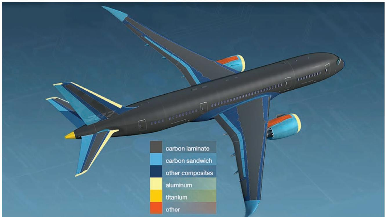
FIGURE 1. Advanced composites used throughout the Boeing 787 account for more than fifty percent of the aircraft body<sup>1</sup>.
